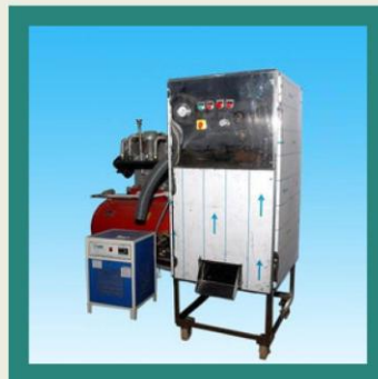
Cashew Peeler Machine (Using Airblasting method)
